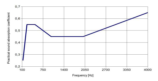
Weighted sound absorption coefficient αw = 0,50 (LH)
