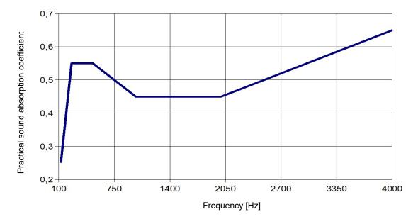
Weighted sound absorption coefficient  $\alpha w = 0,50$  (LH)
